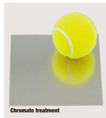
Comparison between chromate and low-gloss treatments
