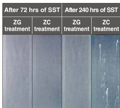
Appearances after salt spray test
