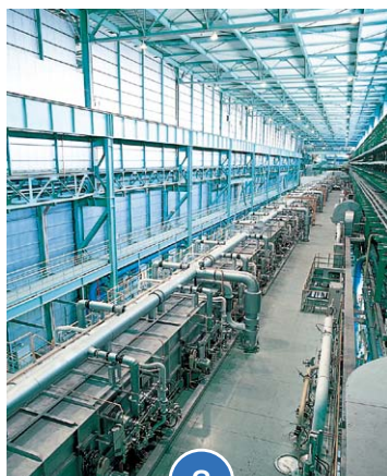
HCGL annealing furnace (Horizontal radiant tube furnace)
