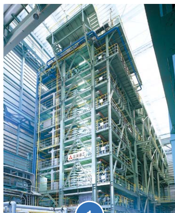
HCGL annealing furnace (Vertical direct-fired reducing furnace)
