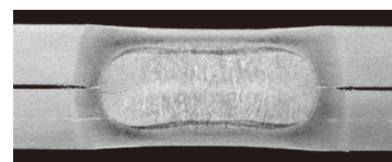
Sectional structure 1.6 mm, coating weight: 70/70 g/m 2
