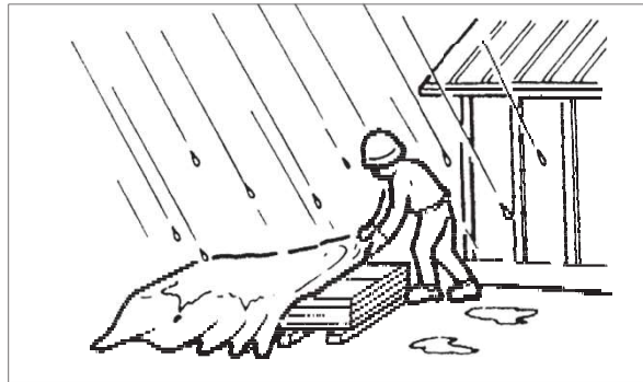
Temporary storage of the panel in an open area
